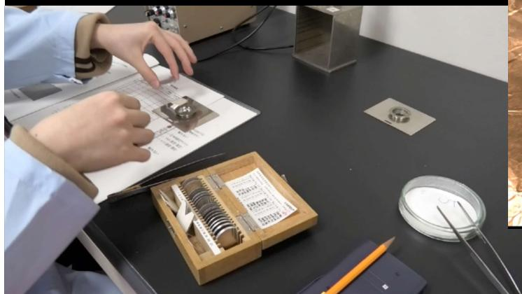
Then, a thicker aluminum plate is put on the source, and the radiation is measured. The measurement is repeated using aluminum plates with different thickness. When the counting rate is low, the measurement time should be prolonged.
