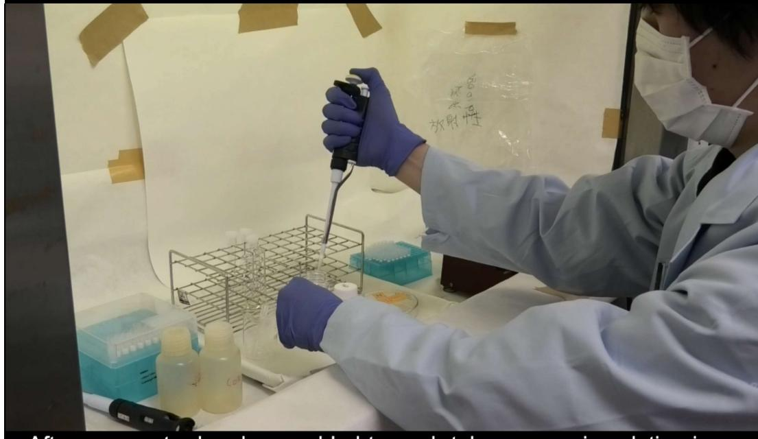
After pure water has been added to each tube, ammonia solution is added gradually. You can observe precipitate formation. Ammonia solution is added until no new precipitate appears.
