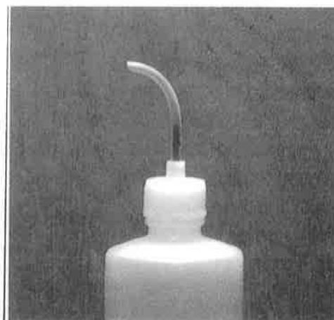
Fig.5 ^{222}\text{Rn} sampler using a wash bottle
