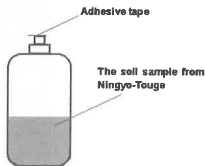
Fig.4 The collection method for ^{222}\text{Rn} -containing air (a simpler method)
