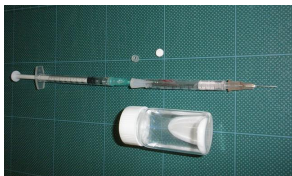
Fig. 1. Manufactured generator assembly with its parts. From bottom to up: adsorbent \text{SnO}_2 powder (before \text{HNO}_3 treatment); Generator connected with eluent syringe; and porous plastic diskette and short end of plastic tube (see text for more detail).
