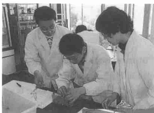
Fix the Kiriya filter paper around GM counter
